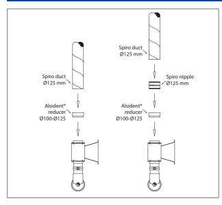
Connection with Alsident® reducer 4-100125 to spiro duct Ø125 mm with and without nipple.
