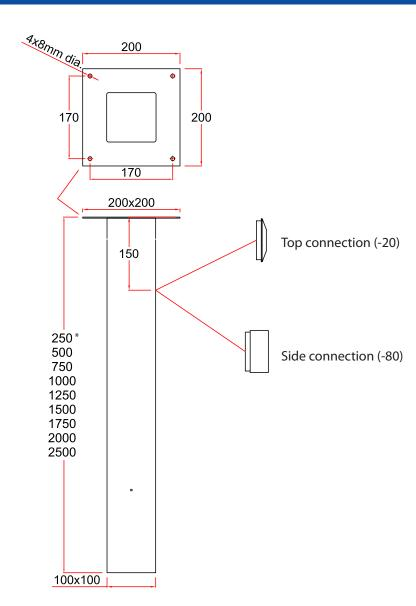
Only for socket pipe with hole (side connection). Hole to be made by installer.
