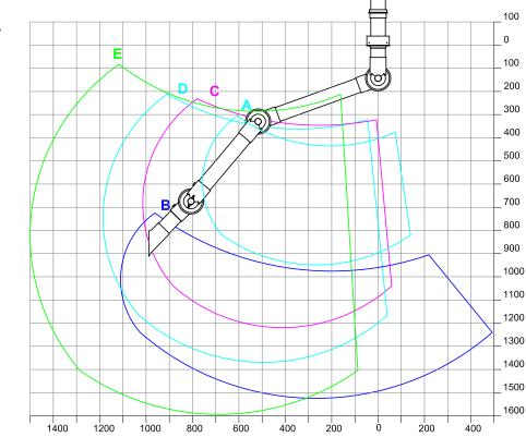
A: Model 63-3535-3-7-5 B: Model: 63-3590-3-7-5 C: Model: 63-5545-3-7-5 D: Model: 63-6555 E: Model: 63-9065-3-7-5
