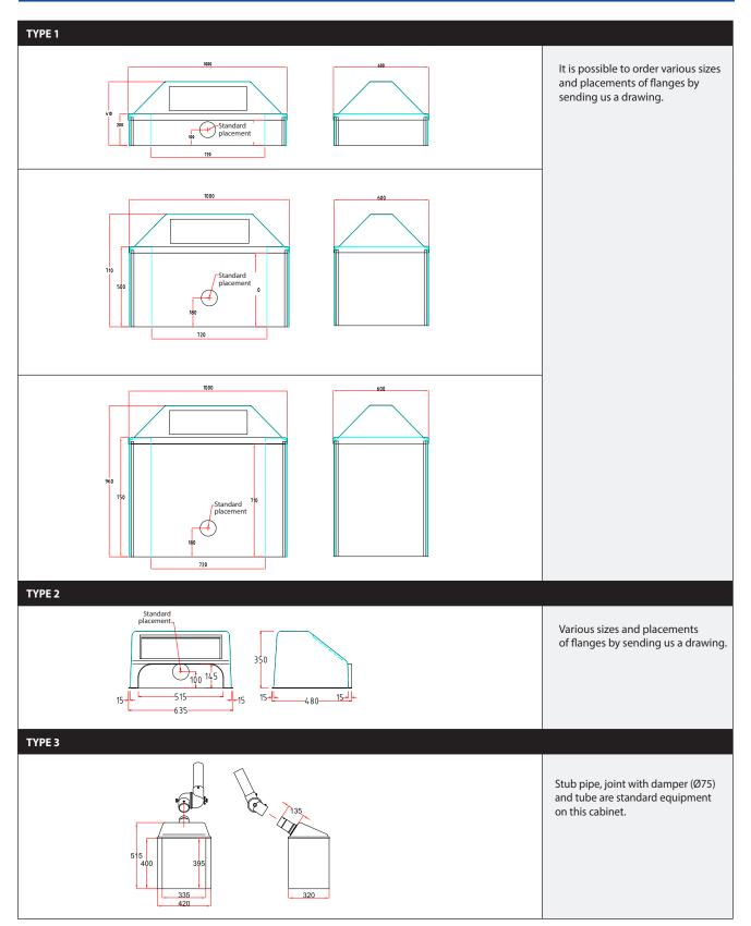
The cabinets are delivered with standard placement of flange unless a special placement is ordered. (all measurements in mm)
