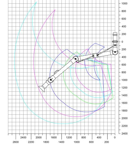
A: Model 100-55-3-6 B: Model 100-4540-3-6 C: Model 100-5545-3-6 D: Model 100-6555-3-6 E: Model 100-9065-3-6\* F: Model 100-10585-3-6\*\*
