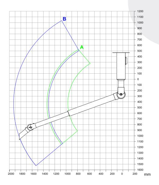
A: Model 900-1300-3 R: 950-1300 mm B: Model 900-1900-3 R: 1300-1900 mm Accessory: Extractor Tube No. 1-7525
