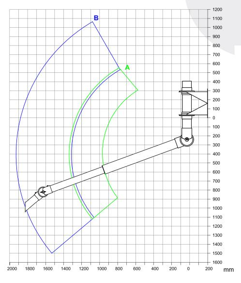
A: Model 900-1300-2 R: 950-1300 mm B: Model 900-1900-2 R: 1300-1900 mm Accessory: Extractor Tube No. 1-7525
