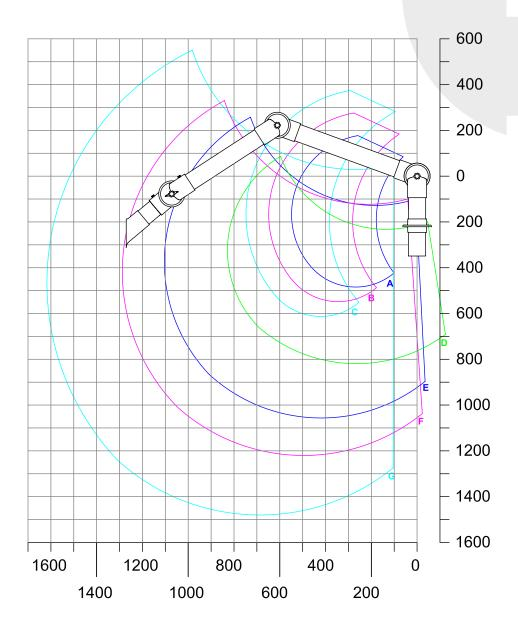
A: Model 75-35-1-7-5 B: Model 75-45-1-7-5 C: Model 75-55-1-7-5 D: Model 75-5335-1-7-5 E: Model 75-5545-1-7-5 G: Model 75-9065-1-7-5 R: 550 mm R: 650 mm R: 750 mm R: 830mm R: 1105 mm R: 1290mm R: 1620 mm Accessory: Extractor Tube No. 1-7525-7-5
